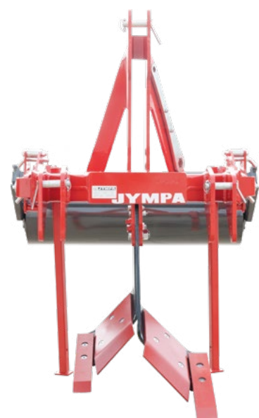
Model MINTAKA-1 with \varnothing 325 mm smooth roller
