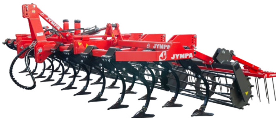
Model OSIRIS-EL-19-2F-PL with swallow-shaped points, elastomer damped tines, Ø 410 mm single cage roller and rake.
